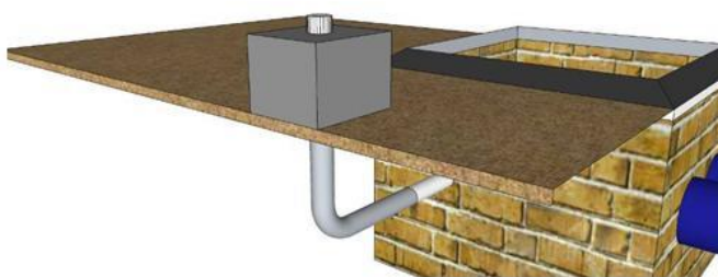
Middle cable entry for goosenecks, camera poles, traffic light poles, barriers, etc.
